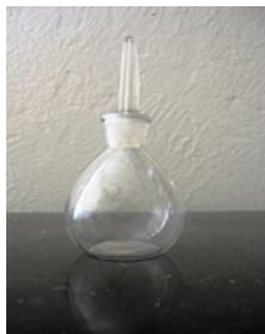
Fig. 2. Pycnometer for density measurement.
