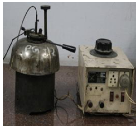
Fig. 6. Pensky–Marten's apparatus for flash point measurement.
