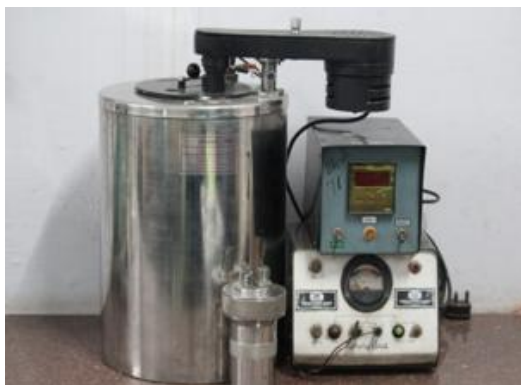
Fig. 12. Bomb Calorimeter for calorific value measurement.
